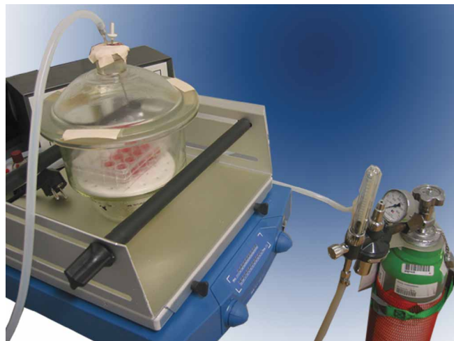
Figure 2 | A 24-well culture plate containing infected tail blood in culture medium, placed in a glass desiccator (candle jar). The infected blood is cultured overnight in the desiccator, which is placed on a shaker and gassed with a gas mixture of 5% CO 2 , 5% O 2 and 90% N 2 .
